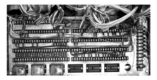
Decisions made by the controller are communicated, via the back panel, to the load switches which are plugged into the load switch bays on the back panel. The load switches then activate the field terminals which turn the signal heads red, yellow, and green. In addition, vehicle detections are input to the controller via the detector amplifiers which are also wired to the back panel.
