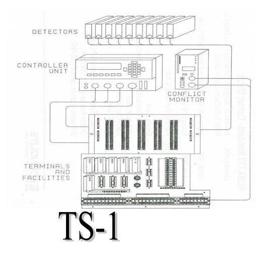
In a TS-1 configuration the controller is connected to the back panel and other cabinet devices via three MS-type connectors designated A, B, and C with designated pin configurations. A fourth D connector may be added to provide advanced features but a standard pin configuration is not specified by NEMA for this connector; it is manufacturer specific.
