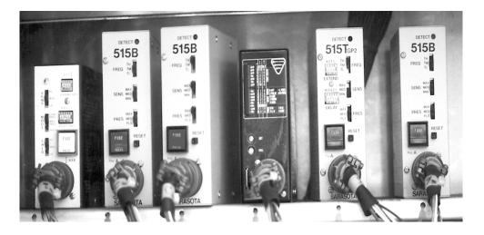
Detector units are referred to as "detector amplifiers" when they are used with inductance loops, which are the most common field units used for vehicle detection. In addition to identifying vehicle actuations based on information received from the inductance loops, the detector amplifiers also power the inductance loops, resonating them at a selected frequency.
