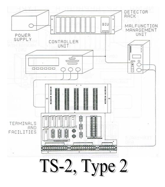
Both the Type 1 and Type 2 configuration make use of a Malfunction Management Unit (MMU) which replaces the TS-1's conflict monitor. The MMU provides the same basic conflict and voltage monitoring functions as a conflict monitor, but with a host of additional features, including:
