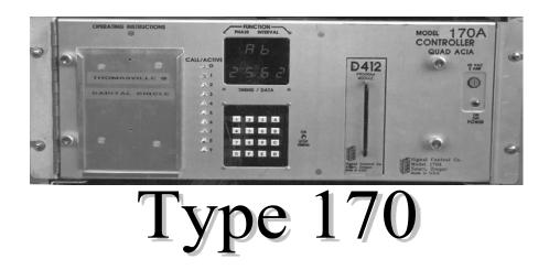
The Type 170 specification results in standardized hardware, which allows a higher degree of equipment interchangeability. In general, equipment from one manufacturer can be mixed-and-matched in a controller cabinet with equipment from other manufacturers, with little or no loss in performance. Since the hardware is standardized, money is saved on spare parts as well as the training of maintenance personnel.
